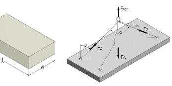
The slab unit has the following dimensions: L = 5 m w = 2 mt = 0.2 m
