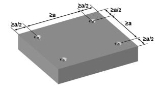
L = anchor length a/2 = edge distance e = cover to anchor head R = recess radius
